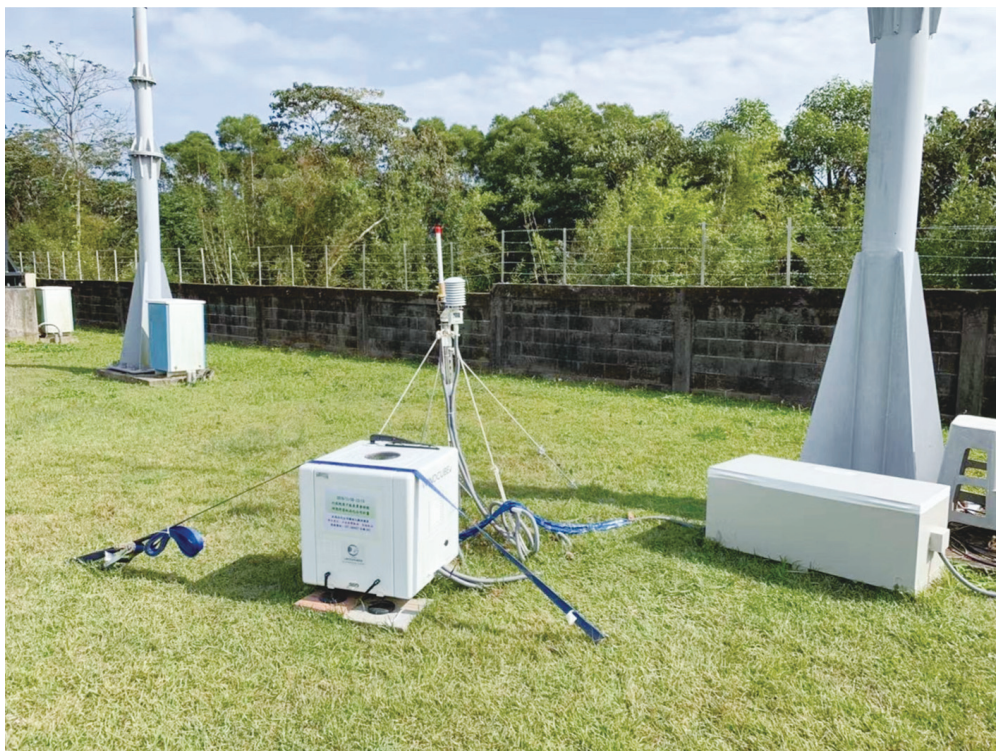
Fig. 4. Employed LiDAR system in INER campus (by author).
