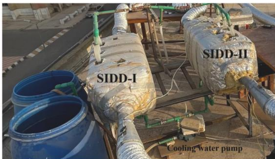
A stage of silica-gel pad and heat exchanger for intercooling
