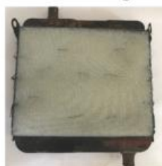
A stage of silica-gel pad and heat exchanger for intercooling
