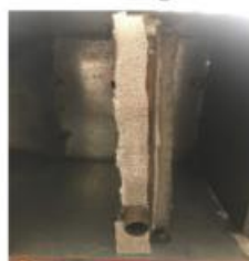
A stage of silica-gel pad and heat exchanger for intercooling
